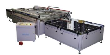
ATMA GS2040 Semi-Automatic Flat Glass Screen Printer
